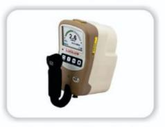
Ludlum Pressurized Ion Chamber Survey Meter (Model 9DP)
