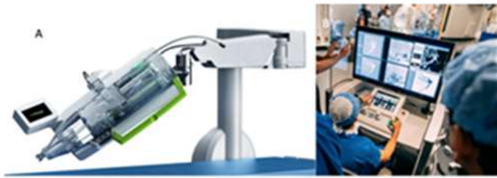
Figure 2: Robotic System CorPath GRX. (A) A robotic arm equipped with a sophisticated cassette. (B) The procedure's configuration. The main neurointerventionist was seated in a radiation-shielded workstation in the angiography room's corner. The team at the patient's bedside included two neurointerventionalists and a specialist robotic technologist who managed the perfused lines and hubs and loaded the devices.
