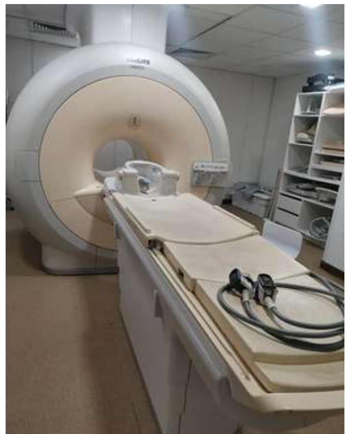
Figure 3 Shows Philips Achieva 1.5T MRI with Dedicated Lumbar spine coil used in MRI
