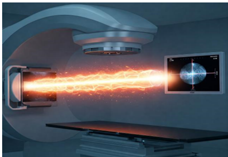
Fig: An organic X-ray sensor is integrated directly into the radiation beam path, transmitting 99.8% of the beam without interruption.
