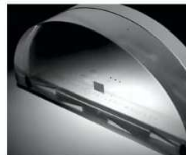
TOMOPHAN® PHANTOM for DBT imaging
