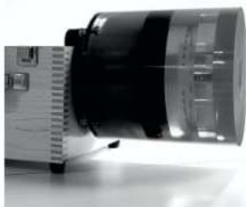
Catphan 500 Phantom for Spiral & Axial CT
